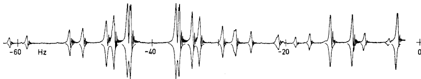
Fig. 2. Part of the observed and calculated ^{19}\text{F} NMR spectrum of neat 1,2-difluoroethane. The spectrum was recorded on a Varian HA-100-15 spectrometer. Each line in the calculated spectrum is assumed to be lorentzian with a line width at half height of 1/4 Hz.
